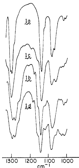
Figure 2. Infrared spectra in the 1350\text{--}1000\text{-cm}^{-1} region of some iron- N -(alkylsulfinyl)alkanesulfonamidato- N complexes, 1 , in Nujol mull.
